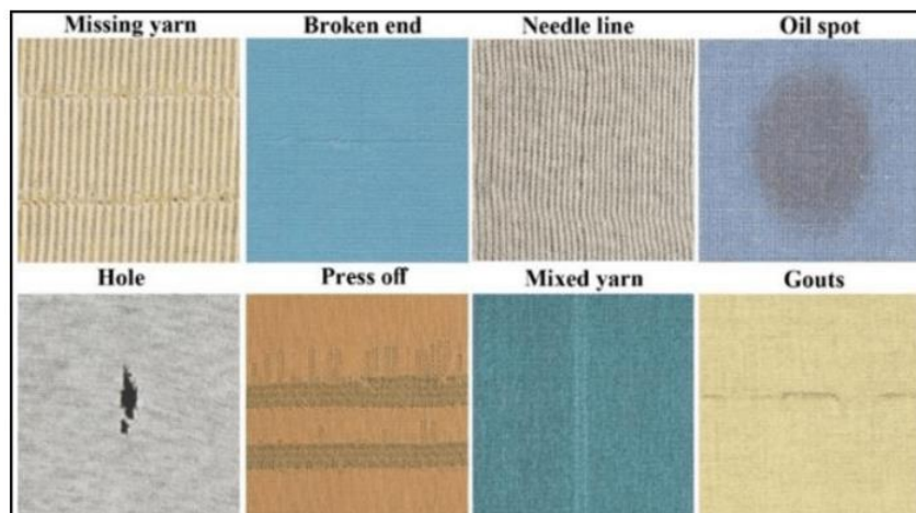
Fig: 2 Samples of defects
